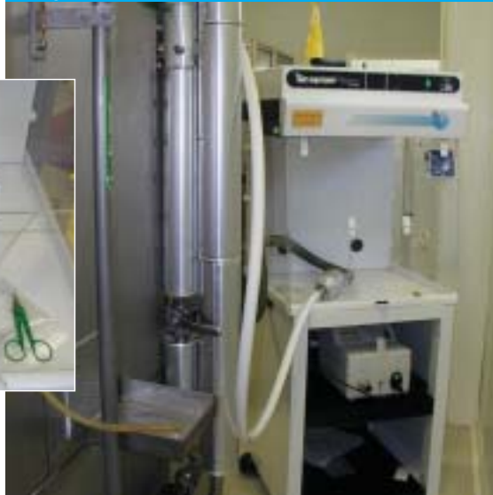
Figure 3 Bottlepack sampling (located at Excelvision) using the PVDF hose, which is connected directly to the filling area.
