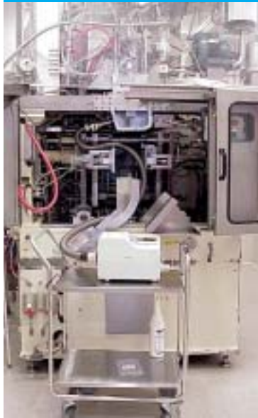
Figure 2 Bottlepack machine (located at Holopack) with the filter holder attached near the filling zone and with the MD8 airscan.
